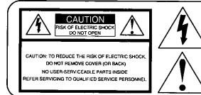
This symbol warns the user that uninsulated voltage within the unit may have sufficient magnitude to cause electric shock. Therefore, it is dangerous to make any kind of contact with any inside part of this unit.
