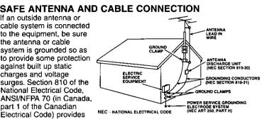
information with respect to proper grounding of the mast and supporting structure, grounding of the lead-in wire to an antenna discharge unit, size of grounding conductors, location of antenna discharge unit, connection to grounding electrodes and requirements for the grounding electrode.
